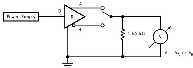
Figure 5. Differential Driver DC Open Test Circuit
