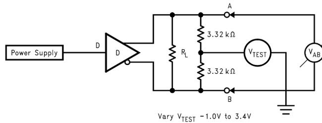
Figure 4. Differential Driver Full Load Test Circuit
